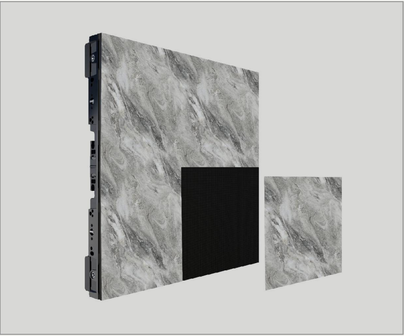
How it goes together: the 500 × 500 mm LED cabinet, the 250 × 250 mm finish panels that clip over its face, and the finished surface. Manufacturer's render.
