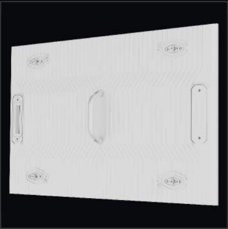
480 × 320 mm die-cast aluminium module, rear with carry handle and fixings. 72 × 48 pixels at 6.67 mm, 60 × 40 at 8 mm, 48 × 32 at 10 mm.
