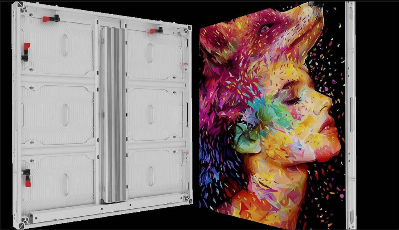
Service side and LED face of the 960 × 960 × 75 mm aluminium cabinet: six modules, the power and data units down the centre, front-release module catches. Product render.
